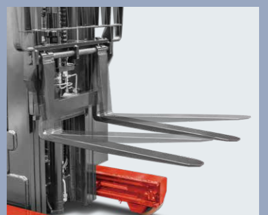
Forks can tilt forward/backward for easy loading
